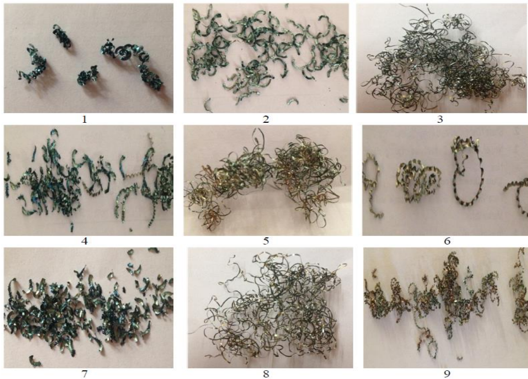
Fig.7 Chip morphology at various cutting speed, feed rate and depth of cut
