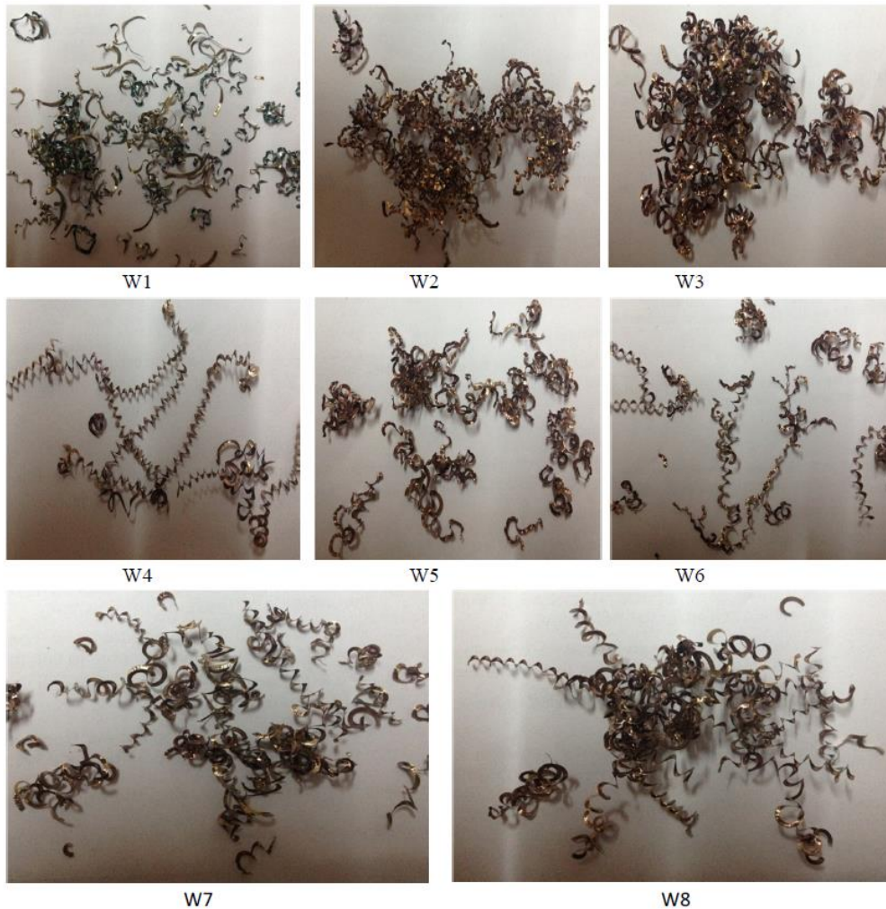
Fig. 8 - Chip morphology at 156 m/min cutting speed, 0.05 mm/rev and 0.2 mm depth of cut and varying cutting length
